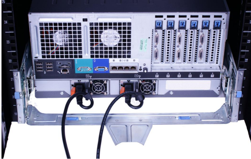
Figure 2: Routing Power Cables Through the Strain Reliefs
